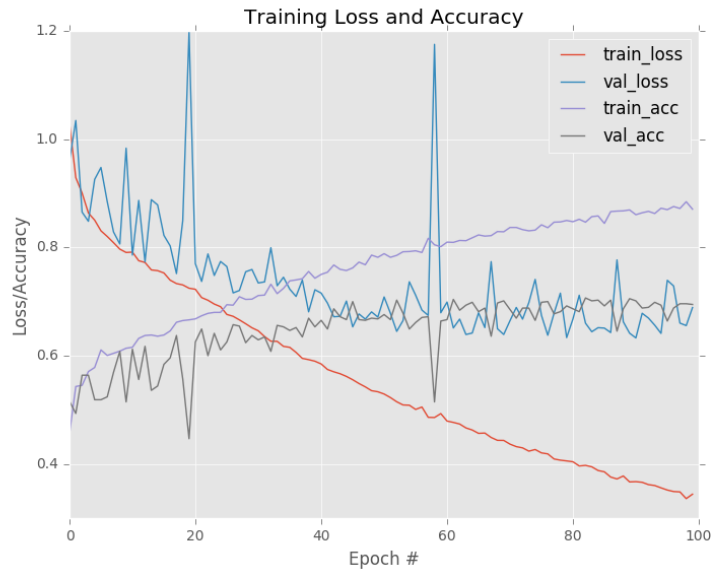
Figure 12.2: A plot of our loss and accuracy over the course of 100 epochs for the ShallowNet architecture trained on the Animals dataset.
